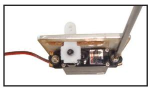
7) Apply 1-2 drops of thin C/A to each of the mounting tabs. Allow the C/A to cure without using accelerator.
