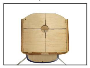
3) Attach the motor to the front of the electric motor box using four 3mm blind nut, four M3x15mm hex head bolts to secure the motor. Please see picture shown.
