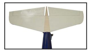
☐ 10) After the epoxy has fully cured, remove the masking tape or T-pins used to hold the stabilizer in place. Carefully inspect the glue joints. Use more epoxy to fill in any gaps that may exist that were not filled previously and clean up the excess using a paper towel and rubbing alcohol.
