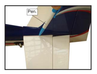
☐ 7) Remove the stabilizer. Using the lines you just drew as a guide, carefully remove the covering from between them using a modeling knife.
